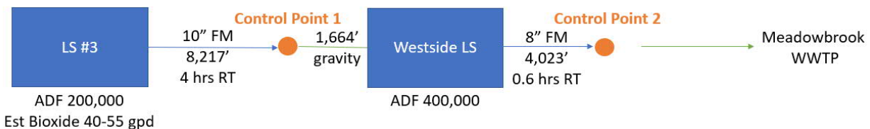
Figure 1 – Simplified line diagram of the Templeton CSD collection system
